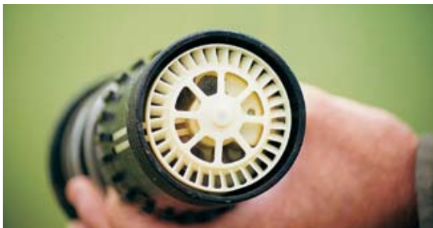
Not a sign of algal growth on sprinkler heads.
